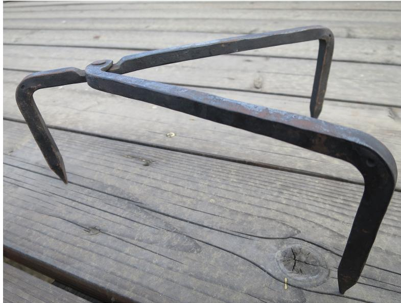
This clever trivet design (from Dave Carroll) folds up neatly to pack with your camping gear, but is sturdy enough for big dutch ovens! Made with tall legs, you can push charcoal under it for cooking; made with scrolled legs, it keeps the hot pot off the table; made extra small, it turns a dutch oven into a cake-baking-oven! The joint requires some careful forging for a smoothly overlapping hinge. Make more than one- everyone who sees it will want to buy it off you!
