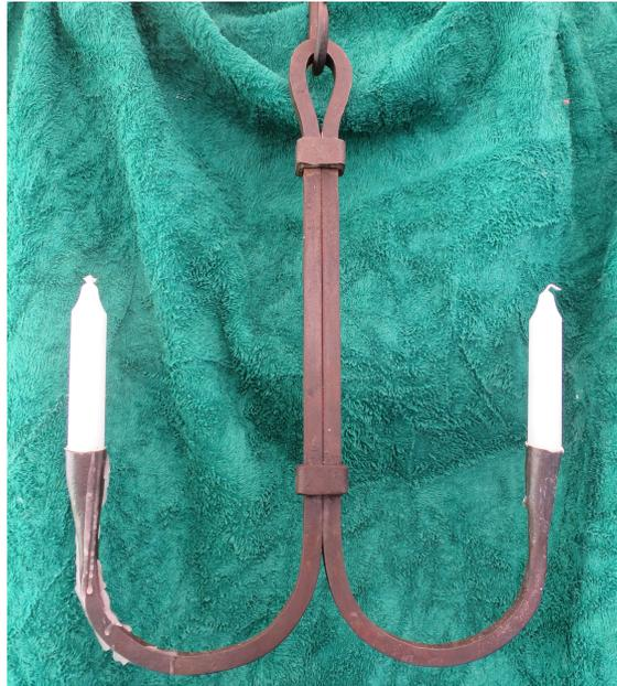
Get an introduction to collaring while forging this olde-fashioned lighting fixture. It'll give your patio that Gothic look! We'll also cover how to use your cross pein to forge bar stock into a sheet metal blank, and how to scroll a round socket through intelligent hammer use (the same method used for making arrowheads, spear, chisels, etc...). Lots of design variations possible, including making it a sconce instead!
