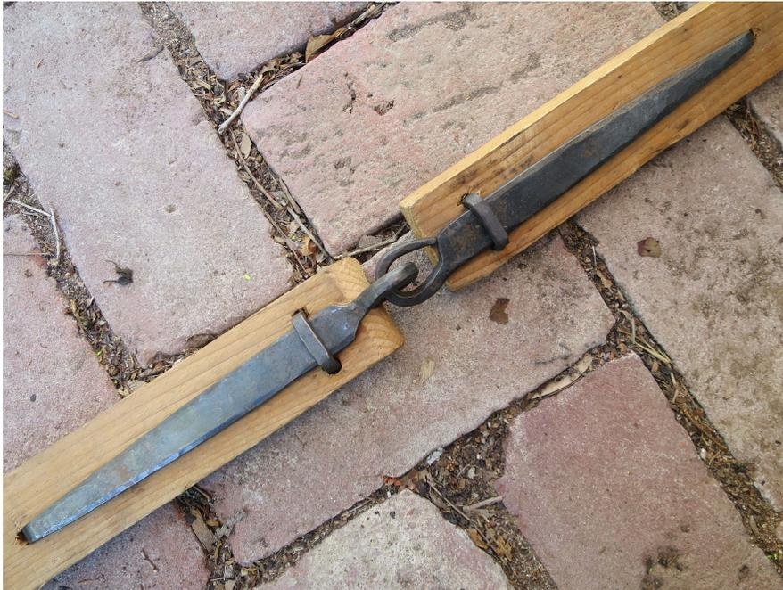
Based on some of the chests found on the spectacular Oseberg ship find, these handsome and functional hinges are a great introduction to connecting two bits of iron in a functional way. And, as an historic twist, we'll learn how to mount hardware with forged staples and 'deadened' spikes (vs. screws...).
