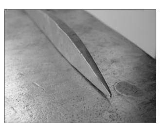
The next step will dictate the shape and size of the finished scroll. Turning the bar on edge, turn a scroll on the end of the bar. I like to start a little way back from the end.
