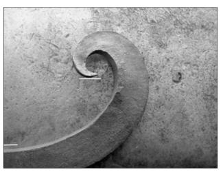
Once the scroll is formedin step 2, decide whether this will be a left or right-handed scroll. This type of scroll has a front and a back, making it one-sided visually. If when you lay it on the anvil face to be beveled, the bar scrolling to the right, it will produce a right facing scroll, and of course visa versa.
