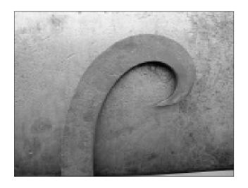
The result of working on the bick is shown above Step 2D.
